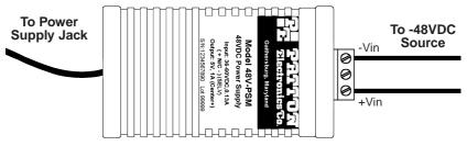
Figure 11. Connecting DC power to the 48V-PSM DC power supply
